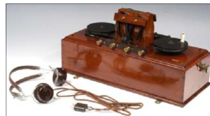
Marconi magnetic detector that received spark telegraphic signals in ships and shore stations. Image courtesy of mhs.ox.ac.uk .
